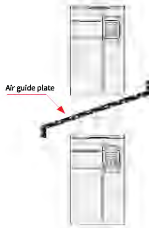
Figure 1-6 Installing one AC drive above another
