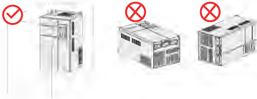
Figure 1-9 Installation direction (T1 to T9 models)
