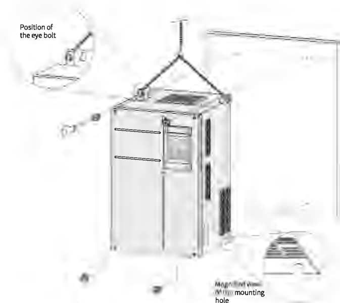
Figure 4-10 Backplate mounting (T7 to T9 models)
