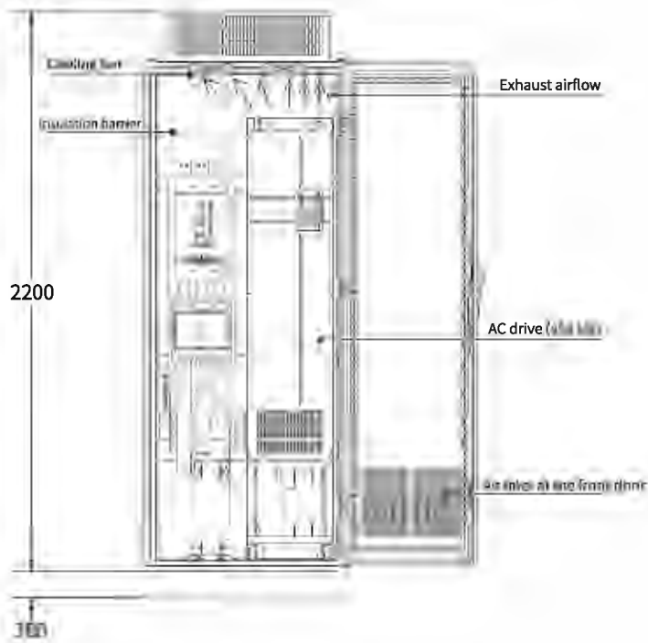
Figure 5-2 Forced ventilated cabinet (with fans on the top of the cabinet)
